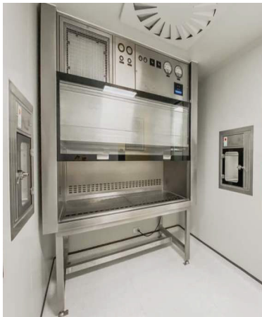
Biological Safety Cabinet Class II
